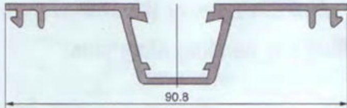
GLAZING ADAPTOR Clips to top of shopfront when glass required both sides
